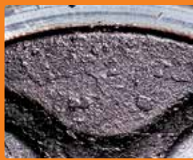
BEFORE: Piston crown with heavy deposit buildup
