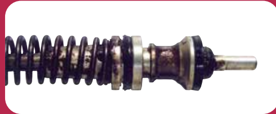
Harmful deposits and varnish buildup—resulting from worn-out, oxidized brake fluid—are apparent on this brake master cylinder piston assembly.
