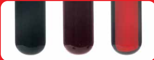
Worn out, oxidized transmission fluid
