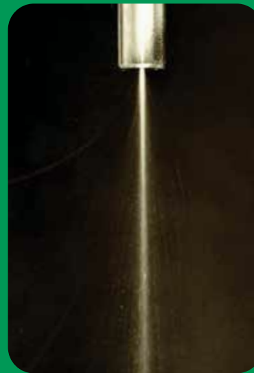
Improper fuel spray pattern resulting from deposit buildup on the diesel injector
