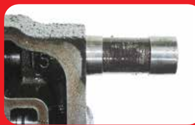
Transmission valve body spool with deposit buildup
