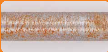
The corrosive effects of ethanol-containing gasoline
