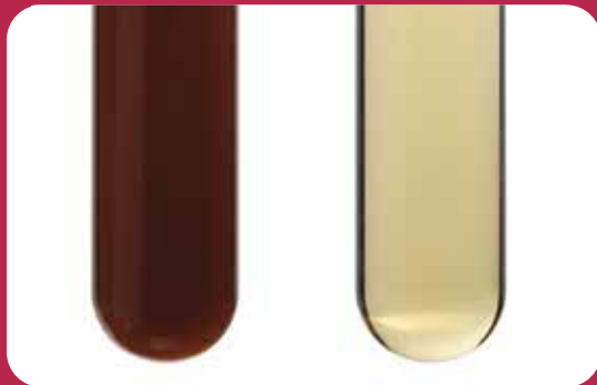
Brake fluid BEFORE (left) and AFTER (right) service.
