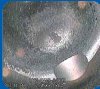
Piston top BEFORE BG Performance Oil Service
