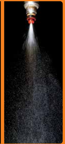
AFTER: A properly functioning fuel injector mists fuel so that the fuel/air mixture is properly balanced and combustion of fuel is thorough.
