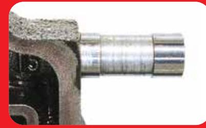
Transmission valve body spool after BG Transmission Service
