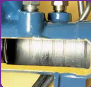
Grooves are worn into the soft metal of the spool valve housing by hardened seals
