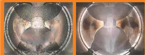
BEFORE: Piston crown with heavy deposit buildup
