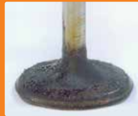
BEFORE: Intake valve with heavy buildup of carbon deposits
